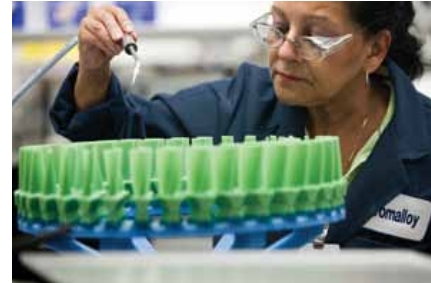
Courtesy of Chromalloy. Wax patterns for turbine engine blade casting.
