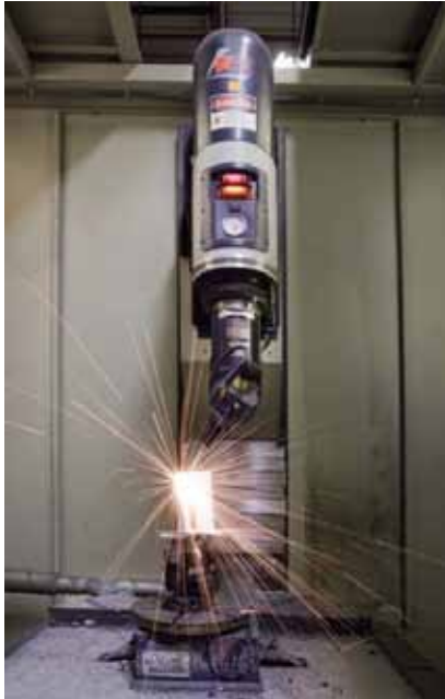
1. Full service. Today's advanced laser drill and shape tools can produce a completed blade by drilling through the ceramic thermal barrier coating applied earlier. Earlier process required the ceramic coating to be applied after the laser drill and ship, causing quality problems. Courtesy: Chromalloy
