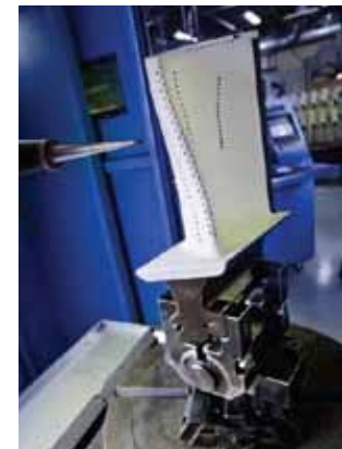
2. Laser hole shaping. The laser can produce shaped and directional holes to manage the cooling air flowing through the blade. This blade has completed its laser drilling and shaping and is ready for a final quality check before shipping. The white portion of the blade is the ceramic thermal barrier coating that protects the blade so that it can operate at higher temperatures. Courtesy: Chromalloy
