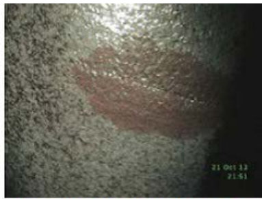
17, 18. Trailing-edge crack is identified in an unflared compressor's upper-half S0 vane using dye penetrant (left); measurement is at right
