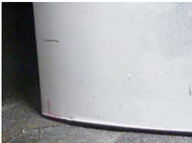
10. Radial tip crack was identified with visible dye penetrant
