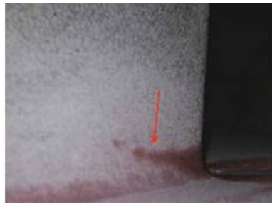
11. Trailing-edge platform crack was found with visible dye penetrant
