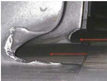
13. Torn metal at trailing edge of S0 vane was caused by tip liberated from the leading edge of an R1 blade
