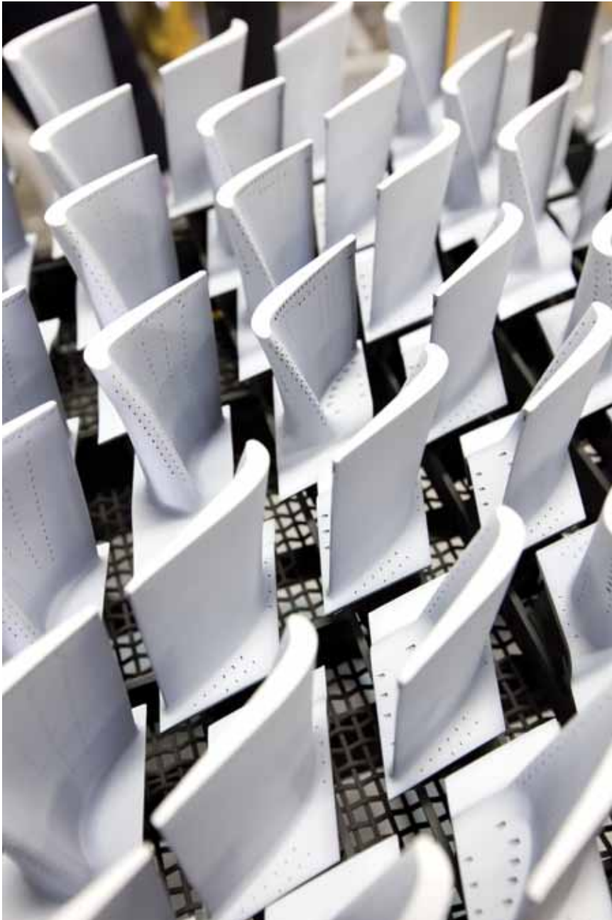
LEFT ◀ Turbine engine blades with Chromalloy coatings.
