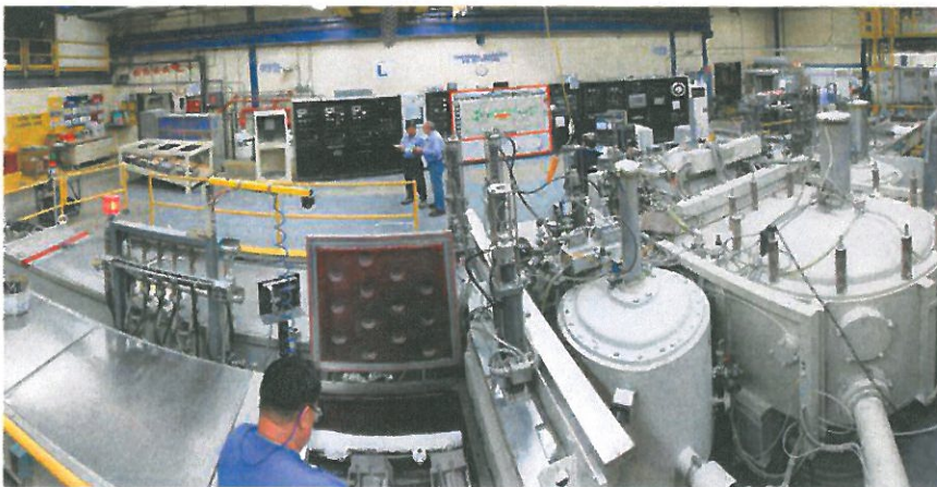
Electron beam physical vapor deposition at Chromalloy facility in Orangeburg, New York.
