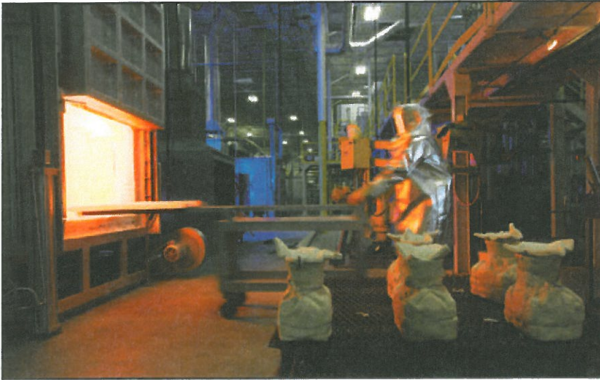
Chromalloy installed larger material handling devices, larger furnaces and larger testing inspection equipment. The company is now equipped to manufacture parts that will fit up to a 122 cm envelope and weigh 68 to 79 kg.
