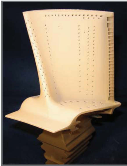
Figure 1. Aerospace turbine engine blade with thermal barrier coating. Ceramic coatings, which are electrically non-conductive, cannot be reproduced by electroplating or anodizing.
