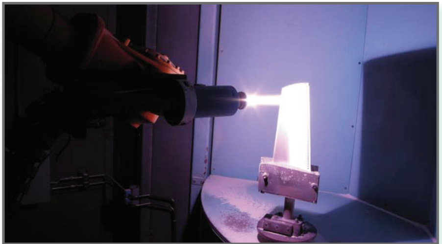
Figure 3. Air plasma spray robot applies thermal barrier coating.
