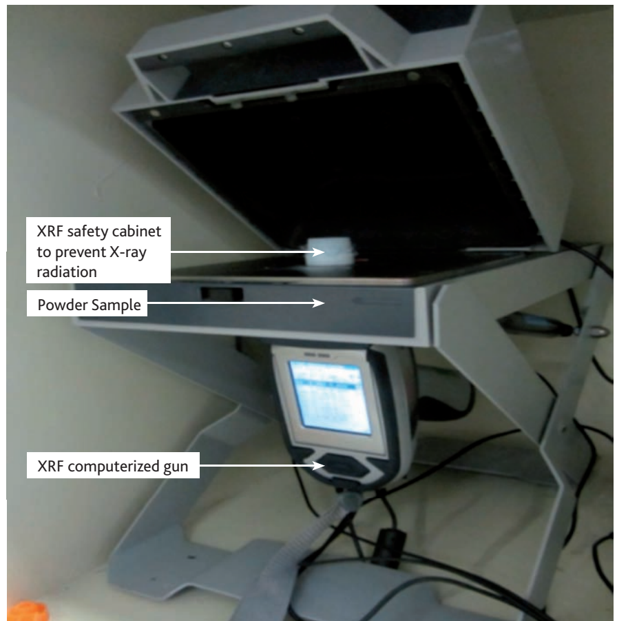
Figure 3. XRF analysis is performed on each lot to ensure the chemical composition meets the customer's requirements.
