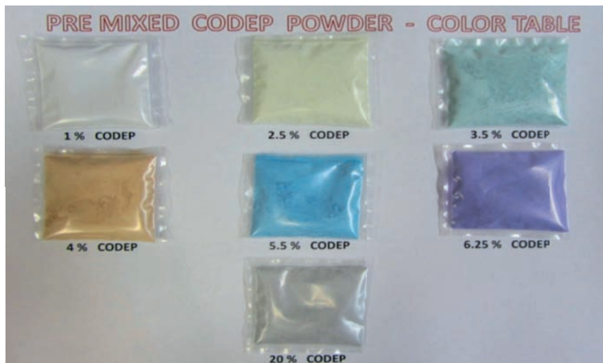
Figure 2. Color pigment identification eliminates human error. Pre-mixed powder can be prepared in a wide mixture composition range with each one identified by a distinct color pigment.
